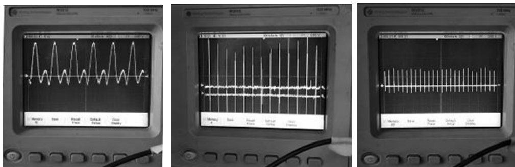
Fig. 2. Characteristic current oscillograms of the electrode systems presented in Fig. 1: a — sum of AC (50 Hz) and DC (100 Hz); b — the sum of DC (100 Hz) and PC (1 kHz); c — the sum of DC (100 Hz) and PC (1 kHz); a ; b — two-electrode system; c — four-electrode system
